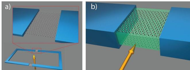
(a) A conventional superconducting quantum interference device (SQUID) consists of a superconducting ring interrupted at two points by weak links (in this case a graphene layer). (b) The new SQUID is made up of a stack of two-dimensional materials, including two graphene layers separated by a thin film of boron nitride. (University of Basel, Department of Physics)
