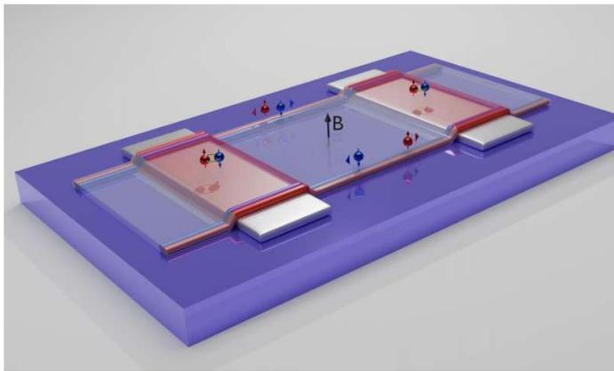
An atomically thin layer of tungsten ditelluride is located between two contacts (in silver). Current only flows through the material in very narrow channels at the outer edges. Credit: Department of Physics, University of Basel
