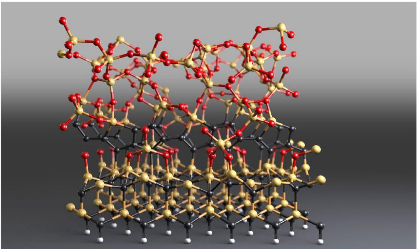
The oxidation process of silicon carbide forms defects: At the interface between silicon carbide (periodic black-yellow atoms) and the insulating silicon dioxide (red-yellow atoms), irregular clusters of carbon rings (irregular black structures embedded in red and yellow atoms) occur. These are bound within the crystal lattice and disturb the current flow. (Image: Department of Physics, University of Basel)
