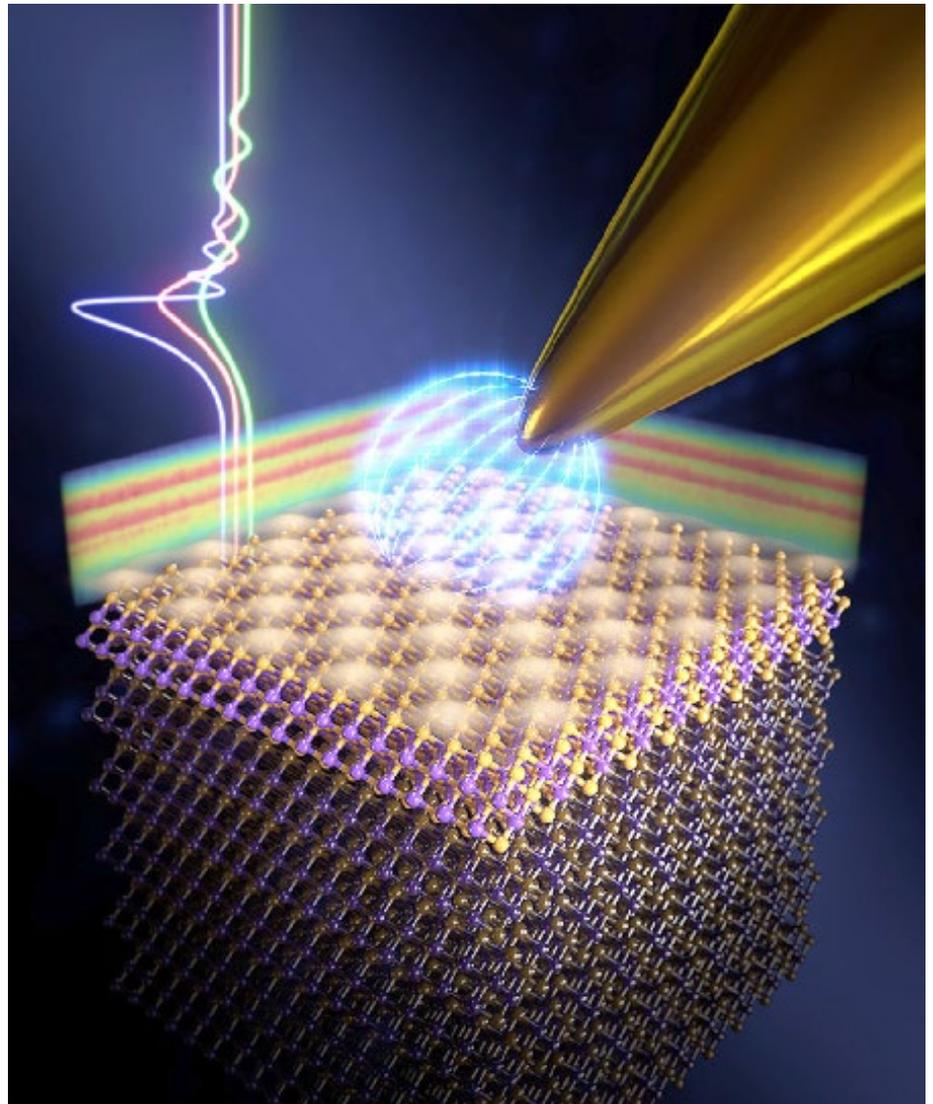
The gold tip is moved across the surface of the topological insulator and experiences energy loss only at discrete, quantized energies (indicated by the curves). This is related to the image potential states (IPS) that are formed over the conducting surface of the topological insulator and are schematically depicted in the background. (Image: University of Basel, Departement of Physics)
