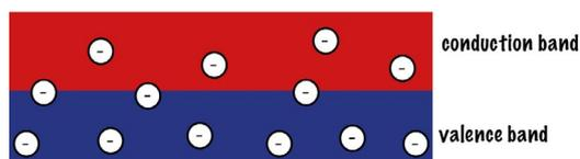
In an insulator, the valence and conduction bands are separated by an energy gap. The energy gap represents the amount of energy that must be supplied to “excite” an electron from the valence band into the conduction band. There is no energy gap in a metal that conducts electricity. As a result, freely mobile electrons are always available and current can flow without the need for thermal excitation.
