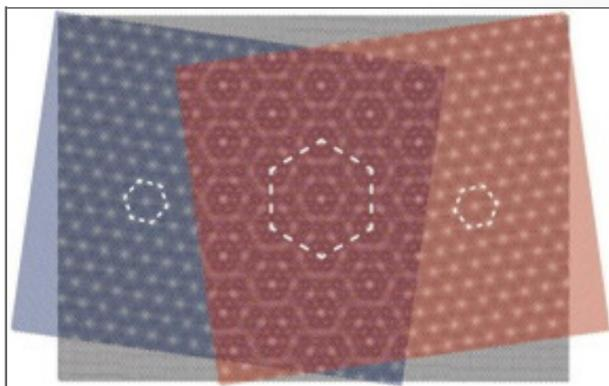
A graphene layer (black) of hexagonally arranged carbon atoms is placed between two layers of boron nitride atoms, which are also arranged hexagonally with a slightly different size. The overlap creates honeycomb patterns in various sizes. CREDIT Swiss Nanoscience Institute, University of Basel
