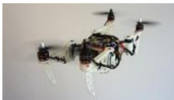
A research team from the University of Zurich has developed a new drone that can retract its propeller arms in flight and make itself small to fit through narrow gaps and holes. This is particularly useful when searching for victims of natural disasters.
