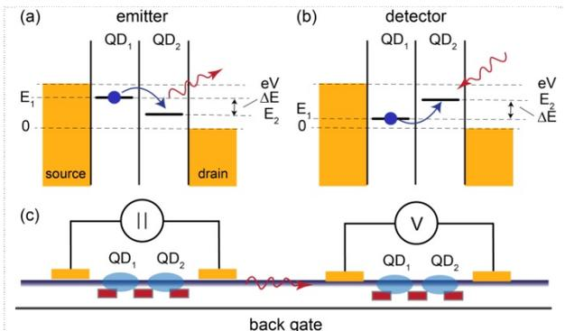
Fig. 1: (a) Schematic illustration of the phonon emission and (b) phonon detection using two coupled quantum dots (QDs) each. (c) Sketch of the envisaged NW device where both a phonon emitter (left) and detector (right) are implemented on a single NW. The back-gate and large electrodes at the contacts (not shown) add a high-frequency short suppressing phonon emission.
