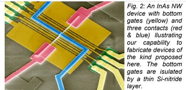
Fig. 2: An InAs NW device with bottom gates (yellow) and three contacts (red & blue) illustrating our capability to fabricate devices of the kind proposed here. The bottom gates are insulated by a thin Si-nitride layer.
