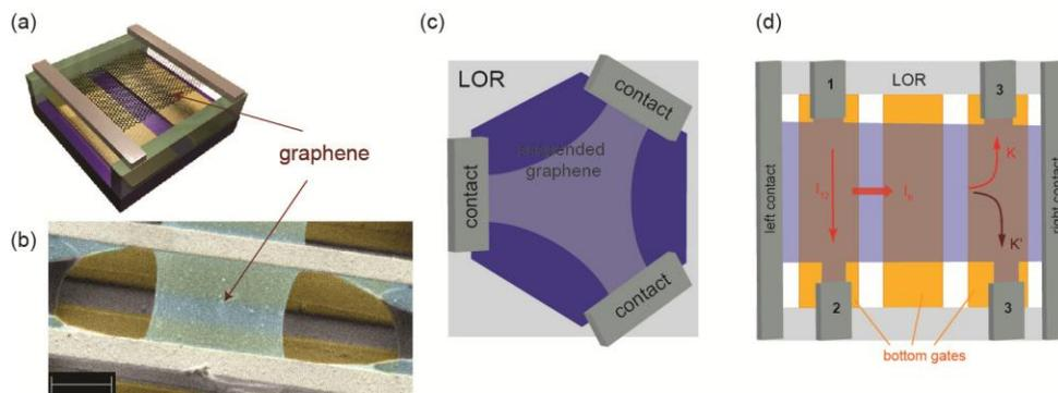
(a) Schematics of suspended graphene and (b) an image of an actual device. (c) One version of shaped graphene that will allow for a trigonal strain pattern ideal for the generation of valley splitting. (d) shows a way to detect valley current using the inverse valley-Hall effect. In this case valley polarization shall arise from either pumping or Hall effect.
