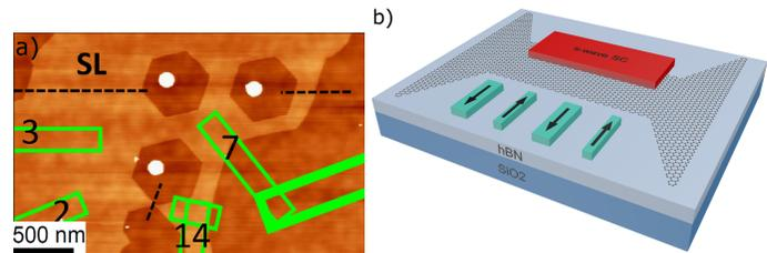
Figure 1: a) Remote plasma fabricated zigzag graphene nanoribbons b) sketch of devices for helical states and majorana Fermions: *armchair* ribbon with nanomagnets (cyan) and s-wave superconductor (SC, red) on hexagonal Boron Nitride.
