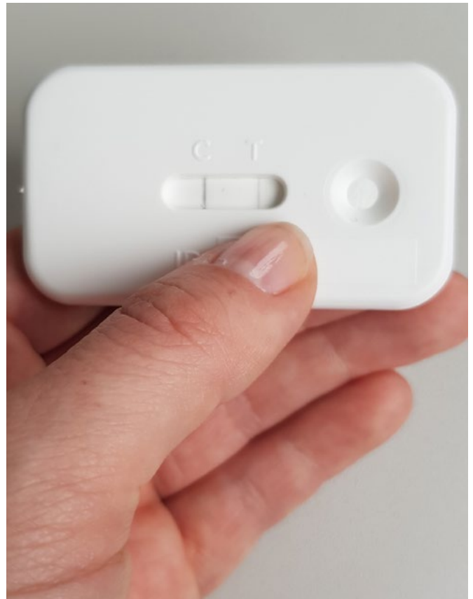
This paper test can be used to detect legionella in water. The left line (C) indicates that the test has worked, while the thin right line is evidence that some legionella were present in the analyzed sample. (Image: Natascha Kappeler)
