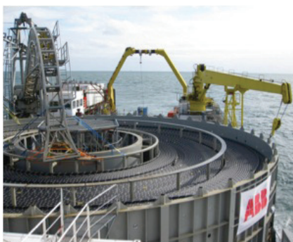
Installation system for submarine high voltage cable (Foto: ABB).
