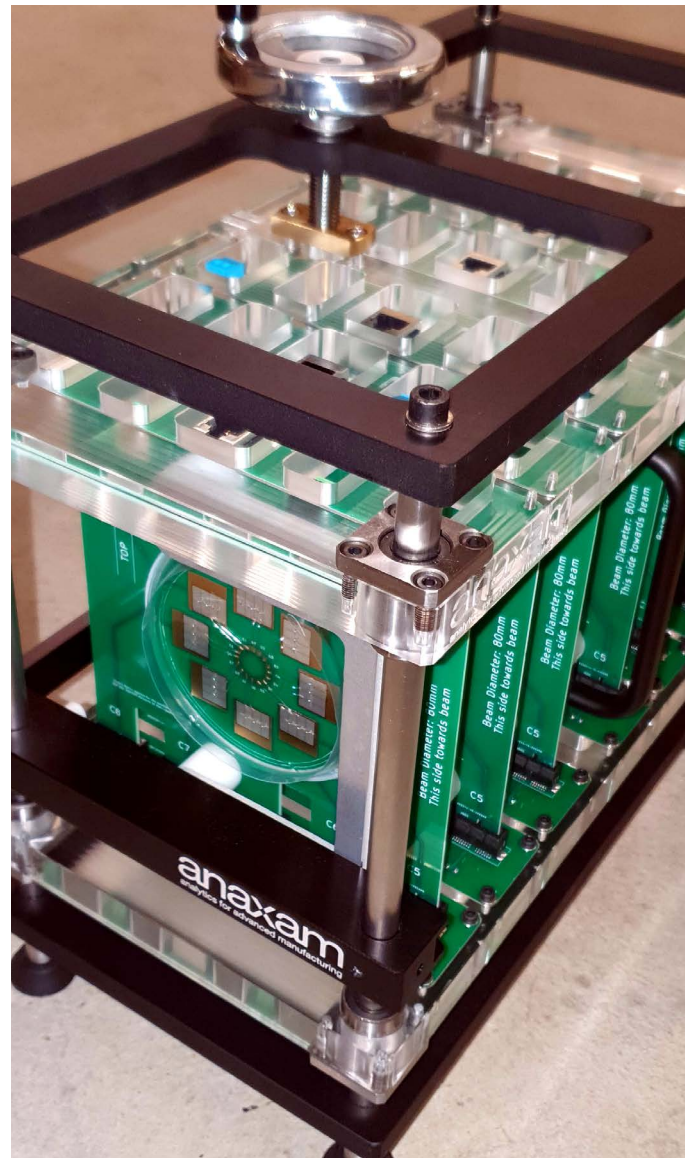
Seen here loaded with semiconductor chips for the planned irradiation experiments, the sample holder was developed as part of the Nano Argovia project CRONOS. (Image: FHNW Windisch)
