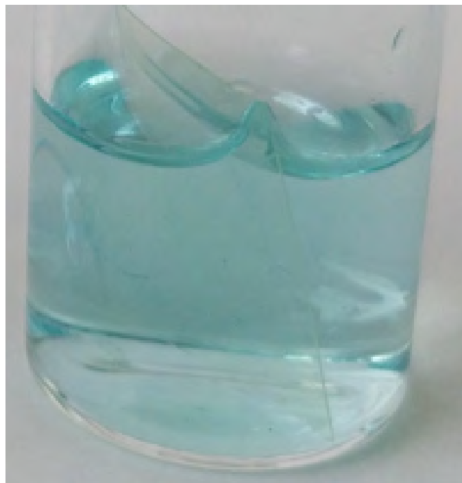
The blue color results from the activity of a model enzyme anchored on the surface (Image: INKA, FHNW).
