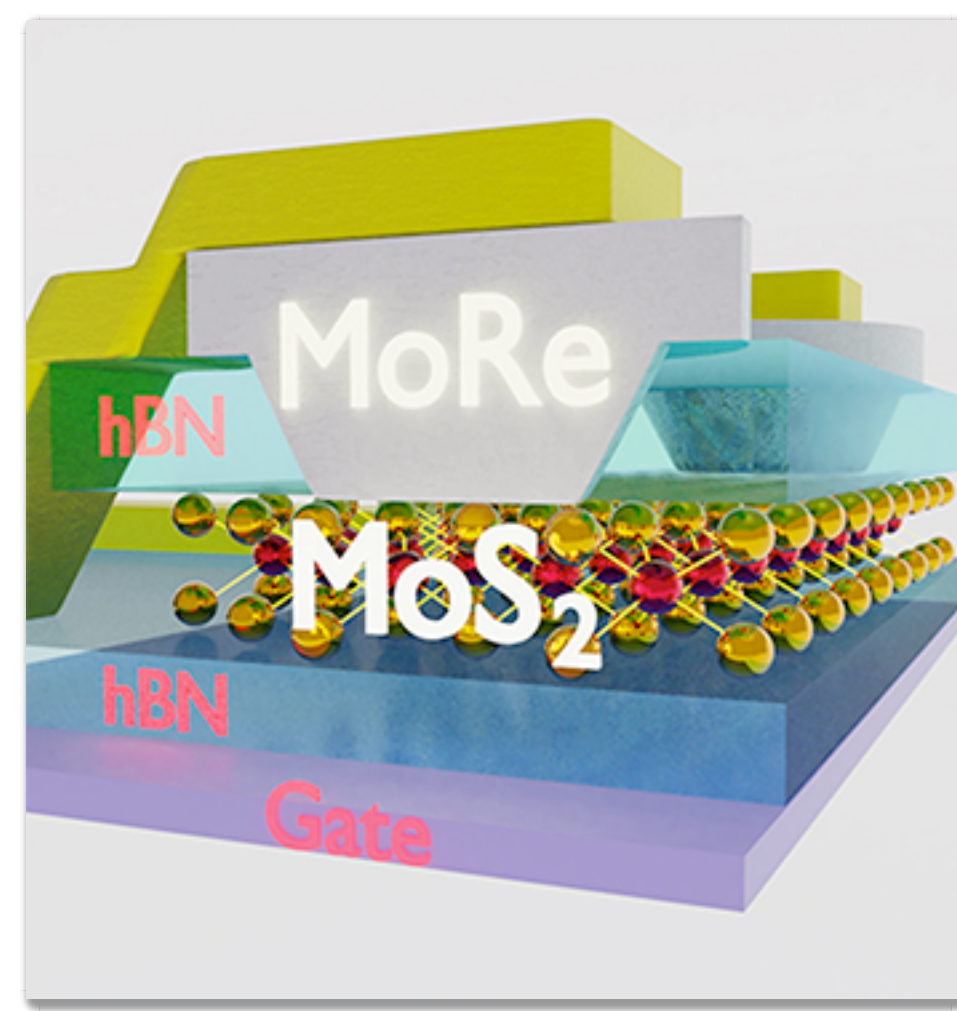
The monolayer of molybdenum disulfide ( MoS_2 ) is sandwiched between two protective layers of boron nitride (hBN), with molybdenum rhenium (MoRe) contacts extending through the upper one. A layer of graphene (gate) is used for electrical control. (Image: Mehdi Ramezani, Swiss Nanoscience Institute, University of Basel)
