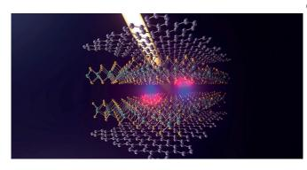
Schematic illustration of the electron-hole pairs (electron: pink, hole: blue), which are formed by absorption of light in the two-layer molybdenum disulfide layer. Credit: Nadine Leisgang and Lorenzo Ceccarelli, Department of Physics, University of Basel
