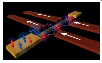
Both quantum dots (dashed ellipses) on the nanowire are tuned by nanomagnets (brown bars) such that they only allow electrons with an 'up' spin to pass. If the orientation of one of the magnets is changed, the current flow is suppressed. Credit: University of Basel, Department of Physics
