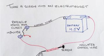
If the electric current is broken, the magnetic field turning the iron core (the screw) into a magnet disappears. The screw loses most of its magnetic force, and the metallic items it attracted before fall back down again. Sometimes, a few of the small magnets in the iron core stay aligned in the same direction, allowing it to retain a small amount of magnetism.
