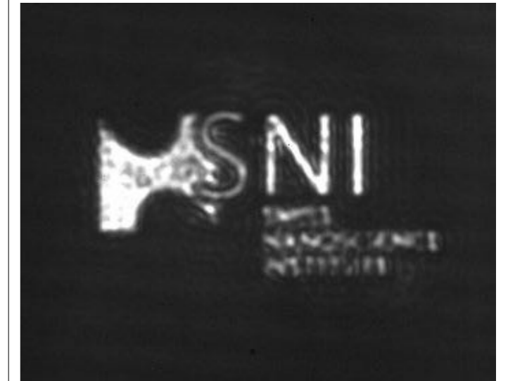
Nanoparticles are trapped in a nano- and microstructure embedded in nano-channels. The depth of the nano/microindentations is 80 nm, and the channel height is 160 nm. (Image: D. Sharma, PSI and University of Basel)
