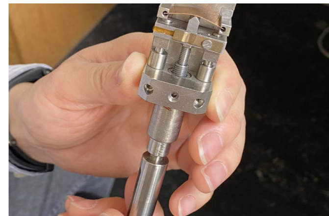
A force from below causes the component to bend, elongating the embedded graphene layer and changing its electronic properties. (Image: Swiss Nanoscience Institute, University of Basel)
