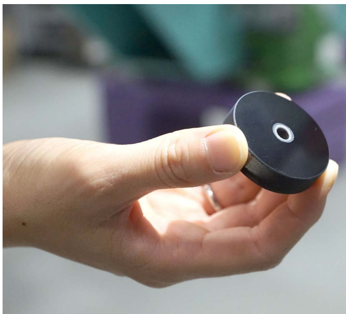
The plasma spray method was used to equip the samples with a ceramic coating that then underwent precise analysis and post-treatment.
