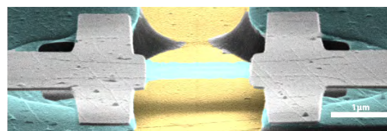
Fig. 3 Scanning electron micrograph of CVD-graphene (blue) freely suspended between two Pd-electrodes (gray). The local Au-bottom-gate is shaded in yellow.
