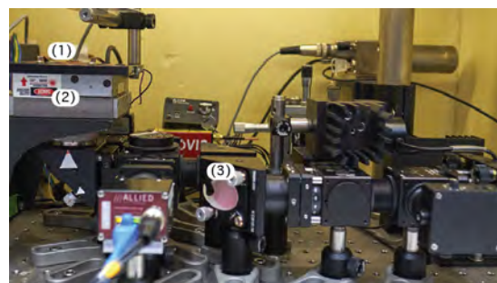
Fig. 4 Set-up modifications to support the new, arrayed nanomechanical sensors (November 2016). (1) New measurement chamber holder; (2) xy-stage; (3) beam shifter to displace detection laser ( LD_{DE} ) relative to the excitation laser ( LD_{EX} ).
