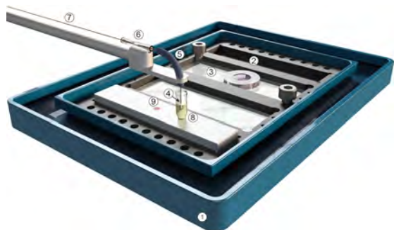
Fig. 1 Live cell imaging chamber, “cell picker” and condition station [1]. The essential components are placed on a work-platform mounted in a live-cell incubator stage (1). For single-cell experiments, miniaturized petri dishes are used to culture the cells (2). These poly-(dimethylsiloxane) (PDMS)-based wells are reversibly bonded to an ITO-coated microscopy slide (3). Cells are lysed by electroporation and the lysate is immediately aspirated (3–5 nl) by a microcapillary (4) [1]. The microcapillary is guided by a conductive sleeve (5) and connected by a press-fit mechanism (6) and a microcapillary (7) to a high precision pump system (not shown). For sample conditioning, the microcapillary tip is immersed in negative stain or trehalose solution contained in a 200 \mu l tube (8). Subsequently, the sample is deposited on a carbon coated EM grid held in place by a groove (9). (Figure and legend adapted from [1].)
