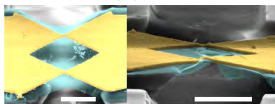
Fig. 2 Scanning electron micrographs of a twin-break junction (golden) on LOR supporting a layer of CVD-graphene (blue shading). Left: Before breaking. Right: The graphene ripped along the line connecting both Au-junctions and reconnected afterwards. Scale bar 2 \mu\text{m} .
