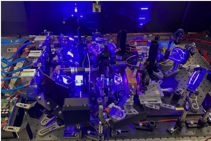
Experimental setup of the femtosecond laser. Blue light is emitted by the new pump diodes. (Image: B. Resan, Institute for Product and Production Engineering at FHNW Windisch)
