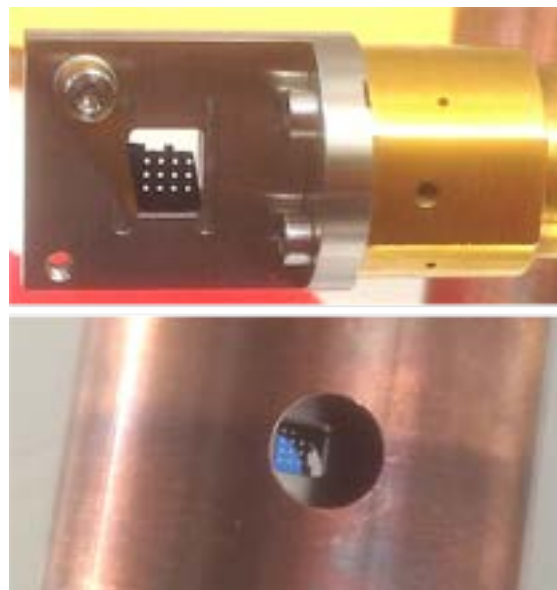
Fig. 3: Top: Membrane chip mounted on a titanium sample holder and bolted to the copper cold finger of a helium flow-cryostat. Bottom: The same membrane inside the copper radiation shield of the cryostat.
