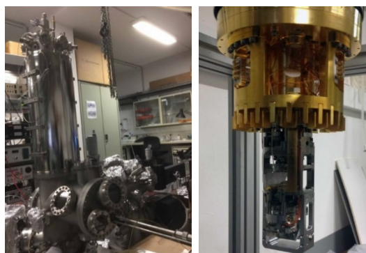
Fig. 1: Overview of the complete set up system (left) and a detailed image of the microscope head (right). At the top wiring and damping system (gold coloured) can be seen. The head itself sitting at the bottom (steel coloured).
