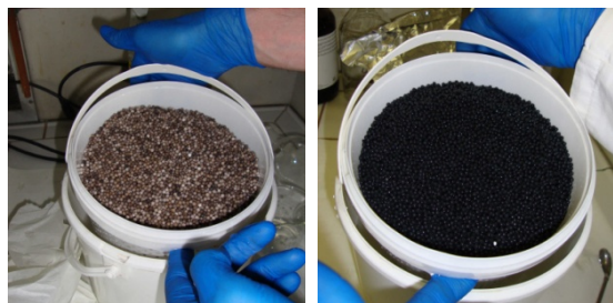
Fig. 3: Coating procedure on ceramic beads by direct impregnation (left, after 20 min ; right, after 2 hrs).
