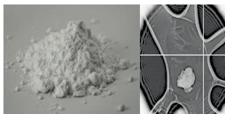
Fig. 1 Grains of icing sugar are cubes of 10\ \mu\text{m} - still 50x larger than the crystals that A3EDPI will look at. The right panel shows an example, about 0.5\ \mu\text{m} across.
