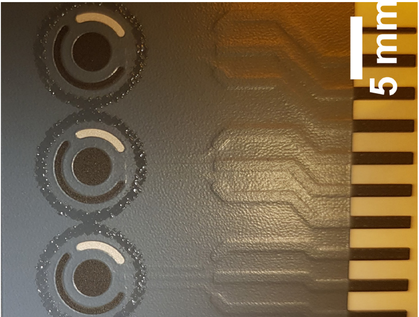
Highly sensitive electrochemical sensor, which is being developed in the PEPS project (Image: CSEM).
